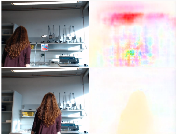
Figure 7. Real World Attacks on FlowNetC. Top: The presence of a printed adversarial patch visible in the centre of the image significantly degrades the optical flow predictions. Bottom: As the patch is covered by the subject, the effect of the patch vanishes.
